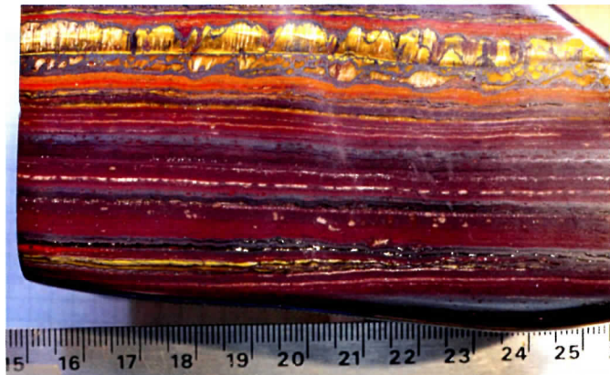
Fig. 4: Hand specimen of Banded Iron Formation, ~2.3 billion years old. The reddish brown-black bands are (ferric) iron ore.
