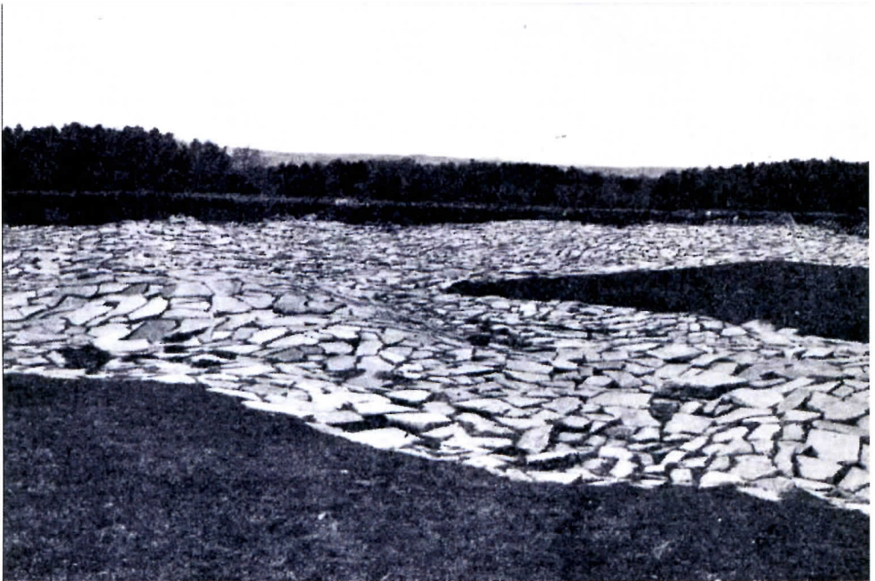
Fig. 3: Slabs of Stonesfield slate laid out in the fields to be split by frost action (from Finberg (1955)).
