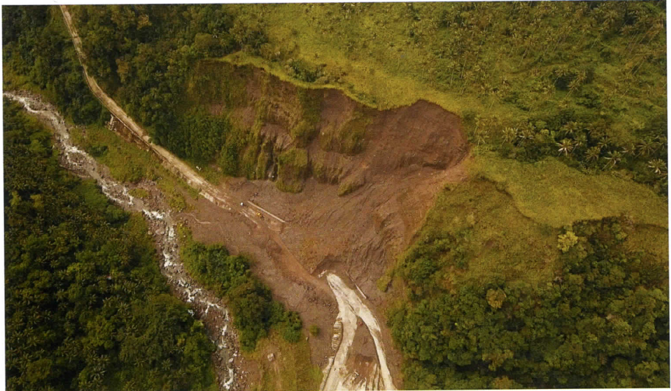
Fig 1: Simple collapse type landslide, which typically occurs where the oversteepened slope is formed of a roughly homogeneous rock type. ( https://www.geotech.hr/en/landslide )
