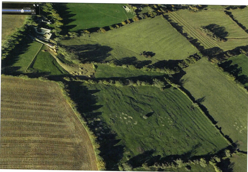
Fig. 6: Arcuate slumps and landslips obscuring Medieval ridge and furrow field patterns, now only visible at the bottom of the field. This shows that the process of slope collapse has been ongoing for hundreds of years. The immediately adjacent field is the location of the 2006 landslide (Fig. 4). View is to the NW.
